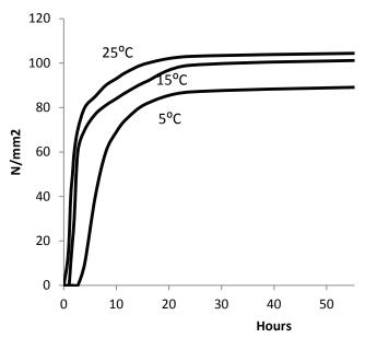
Note: The performance of Nitomortar PE winter grade at  $5^{\circ}$ C is similar to that of the standard grade at  $20^{\circ}$ C.
