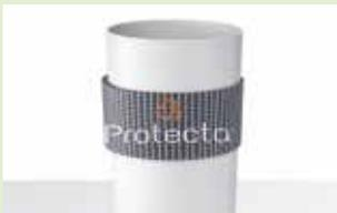
ASF Pipe Wrap contains a graphite material, within a flexible plastic sleeve that reacts to heat; expanding to fill the void created by the melting plastic through-penetration.
