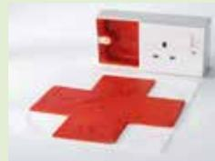
ASF Socket Box Protection Pads are an easy to apply fire and sound rated sealant supplied as a non-setting putty. The pad is hand workable, re-useable and re-serviceable due to its non-setting properties.
